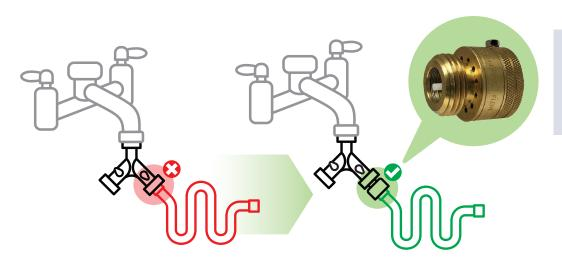
An Atmospheric Vacuum Breaker (AVB) must be used when connecting a hose to a two-way splitter installed on a mop sink.
