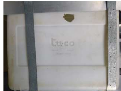
Unapproved hole inlet for filling
