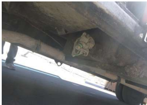
Towel used to plug the wastewater tank.
