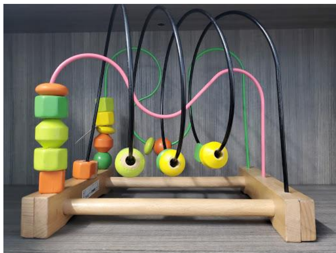
Figure 9. Children's Bead Maze Toy with 528 PPM Lead in the Green Wire, exceeds the 2008 CPSC Lead Limit of 90 PPM
