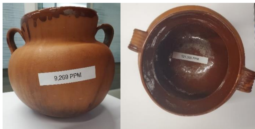
Figure 7. Traditional Bean Pot with over 9,00 PPM of lead outside and over 520,000 PPM of lead inside
