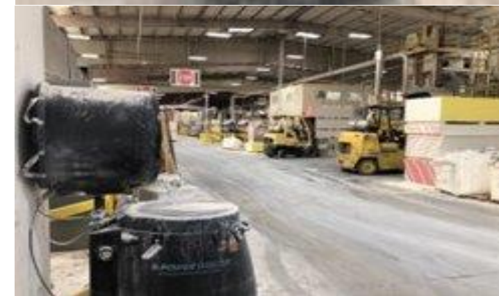
Contaminated Misting System at Job Site
