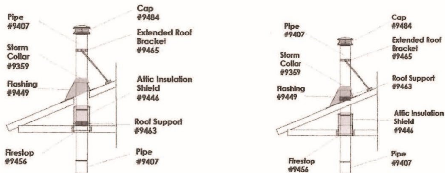
DRAWING 3-5 & 3-6 CHIMNEY INSTALLATION LAYOUT
