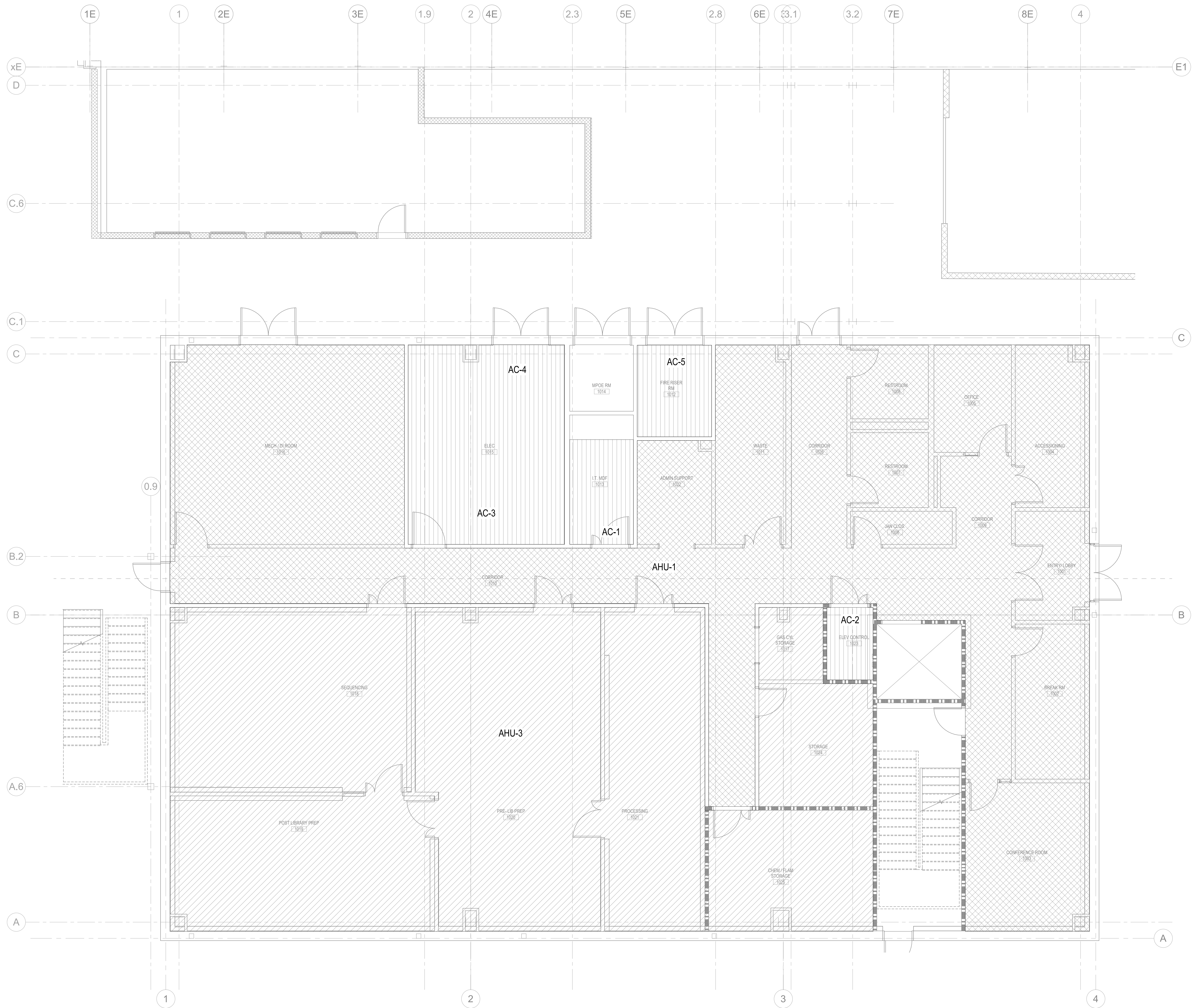
1 LEVEL 1 - HVAC ZONING PLAN SCALE: 1/4" = 1'-0"
